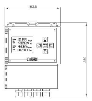
VLW90M Level, open channels flow and pumps control unit
